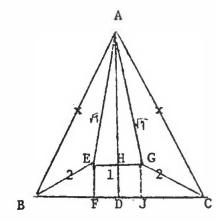
Construct the altitude AD , thus bisecting EG at H . Then  $\overline{\text{HG}} = 1/2$  ,  $\overline{\text{AG}} = \sqrt{7}$  and by Pythagoras' Theorem applied to  $\triangle$  AHG we have
