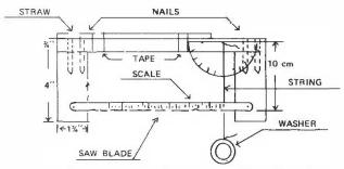
Use the above drawing to construct the clypsometer.
